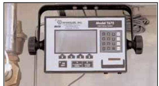
The Sponsler T675 flow meter (above) is included with all CryoMaxx LDV Models.
