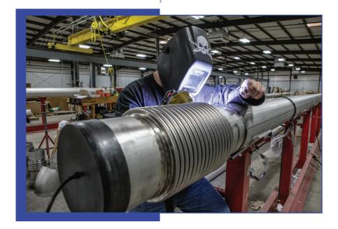
Our manufacturing team builds Vacuum Jacketed Piping using trained personnel and certified welders. Our technicians are highly trained in vacuum technology, insulation techniques and VJP system testing.
