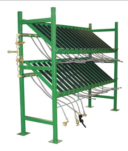
Acme Cylinder Charging Manifolds are designed to provide simple economical filling of up to 60 cylinders at one time. The vacuum and vent controls are located directly on the manifold, eliminating the need for a separate panel. The manifold is provided with a threaded end for future expansion.
