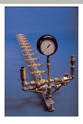
Acme Cylinder Charging Manifolds are designed to provide simple, economical filling of 24 or 48 cylinders. The vacuum and vent controls are located directly on the manifold, eliminating the need for a separate panel. The manifold is provided with a threaded end for future expansion.
