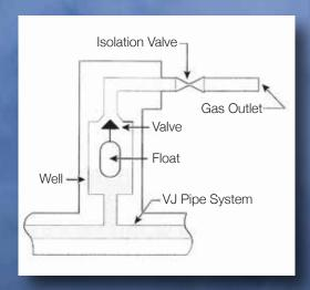
The Mechanical Keep-Cold device allows gas to rise in its vertical well and be vented to atmosphere through a valve. As the gas is vented from the VJ piping the liquid will raise the mechanical float valve and stop the venting. This system maintains the liquid at a constant level in the VJ piping.
